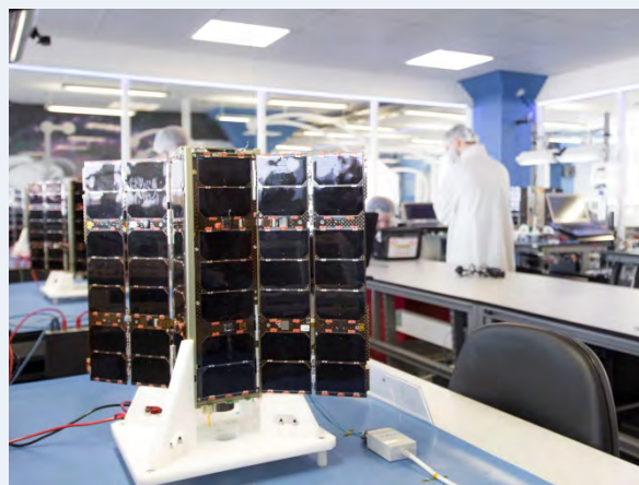
Exhibit 88: Spire's Lemur 2 on a table during testing
