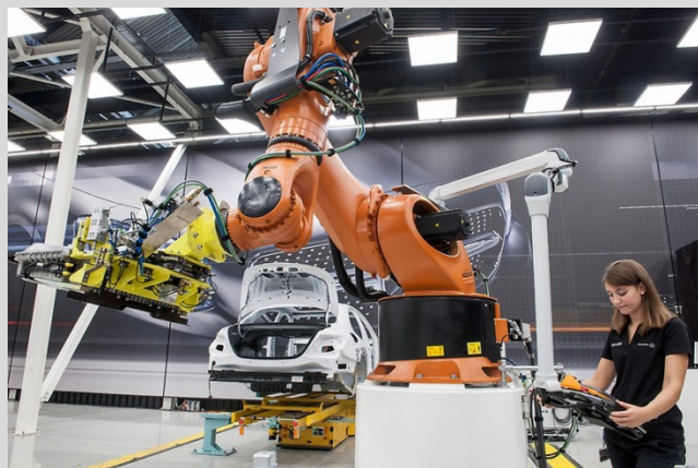
Exhibit 13: The use of individual production cells and AGVs makes assembly more flexible
