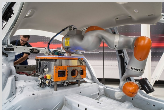
Exhibit 14: A Kuka cobot working inside a Daimler car while humans work from the outside
